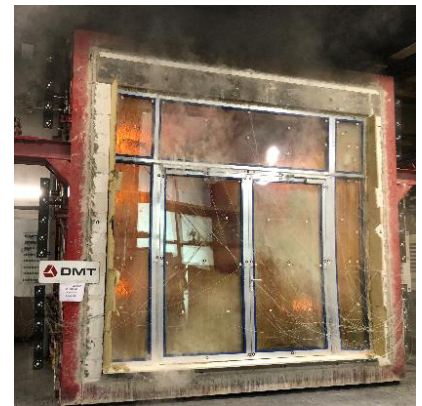
In the first minutes of the fire the protective layer in the glass reacts and turns opaque. This blocks the heat and helps to reduce panic by obscuring the flames from view.
