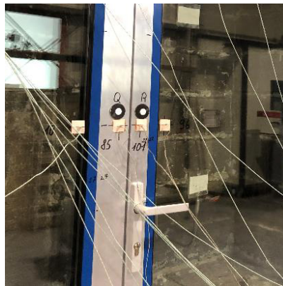
Thermocouples installed all over the test element monitor the surface temperature increase.
